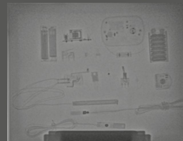
Penetration of 20mm of steel from 80cm distance with 10 pulses using DR panel and XRS-3.
